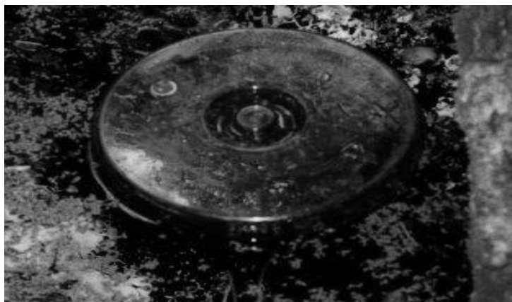
Fig.4. Floating chamber (for collecting gas samples) on the surface of Moszne lake.
