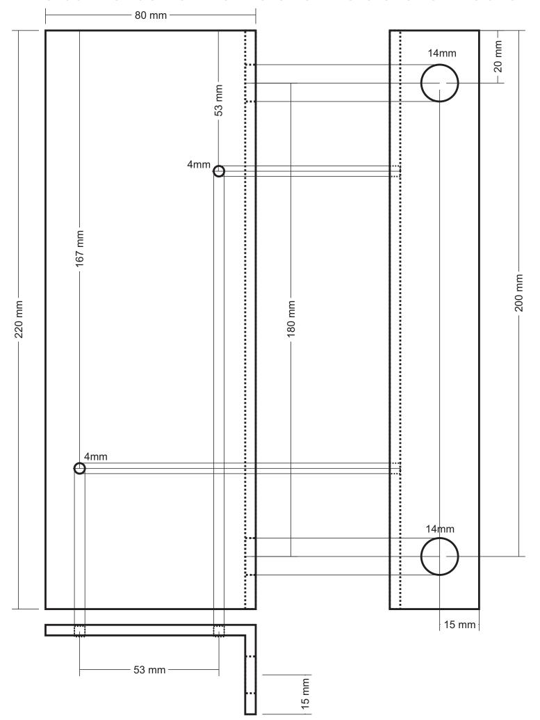
control box of the motor of the elevation tracker
