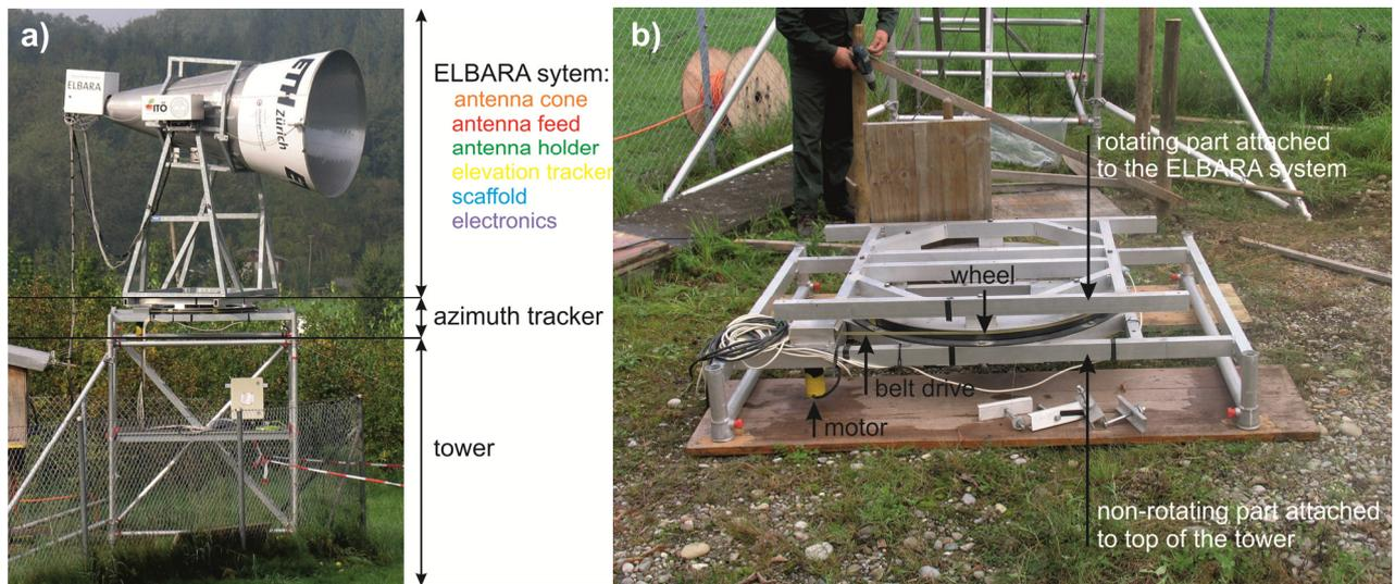
**Figure 1:** a) ELBARA attached to the beneath azimuth tracker and mounted on a small tower. ELBARA system components indicated correspond with Figure 3. b) Close-up of the azimuth tracker used in the earlier experiments [1, 2].
