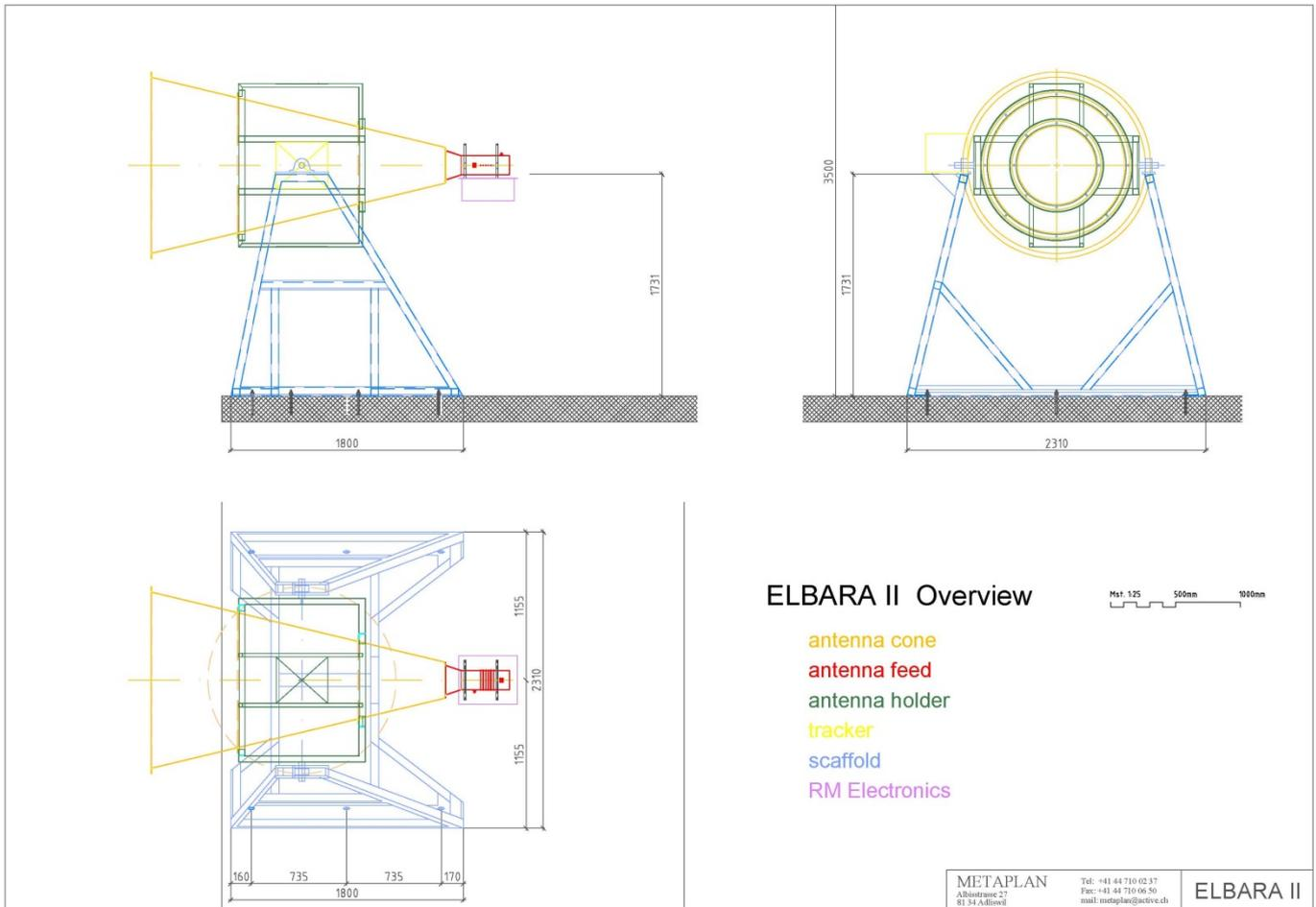
**Figure 3:** Drawings of the entire ELBARA system (without the beneath azimuth tracker) showing its major mechanical components produced by GAMMA (antenna cone, antenna feed, antenna holder, electronics) and IA-PAS (scaffold, elevation tracker).
