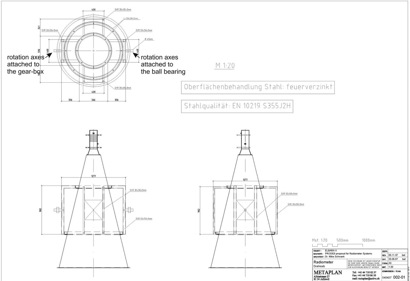
**Figure 7:** Mechanical drawings of the system components provided by GAMMA (antenna (cone, feed, holder), radiometer electronics) and IA-PAS (scaffold, elevation tracker). The ball bearing and the gear-box holding the rotation axes will be screwed to the top mounting plate of the scaffold during the assembly of the ELBARA system in Poland to avoid manufacturing tolerances.
