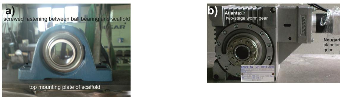
**Figure 6:** Fotos of the ball bearing (panel a) and of the gear-box (panel b) consisting of the Atlanta and the Neugart gear. The ball bearing and the gear-box are screwed on the top plate of the scaffold (Figure 4) during putting together the GAMMA components (antenna (cone, feed, holder), radiometer electronics) with the IA-PAS components (scaffold and elevation tracker) in Poland.
