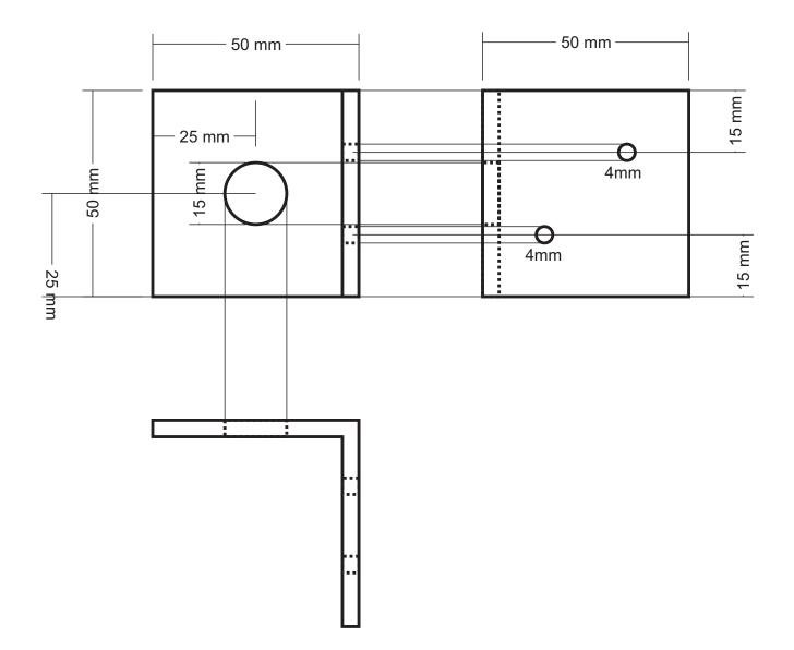
counter-part of inductive switch with mounting angle
