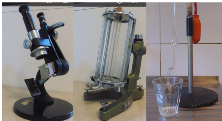
Fig. 2. The used equipments (refractometer, viscosimeter, stalagmometer)
